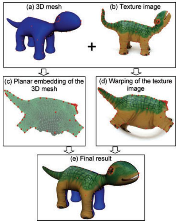
**Figure 1:** Overview of the texturing method: 3D mesh (a) and texture (b), unconstrained planar embedding of the mesh (c), warping of the texture image to match the features with those of the unconstrained planar embedding (d), final textured model (e).
