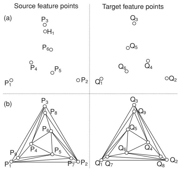
**Figure 11:** Let two sets of feature points  $S_1 = \{P_1, P_2, P_3, P_4, P_5, P_6\}$  and  $S_2 = \{Q_1, Q_2, Q_3, Q_4, Q_5, Q_6\}$  (a); the construction of the compatible triangulation of  $S_1$  and  $S_2$  requires adding 3 Steiner vertices  $\{P_7, P_8, P_9\}$  and  $\{Q_7, Q_8, Q_9\}$  for each set.
