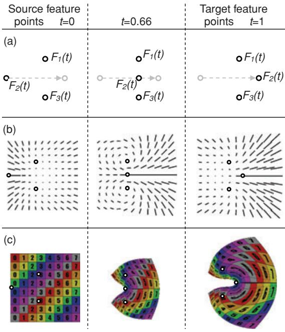
**Figure 4:** Vector-field based warping: linear interpolation of the position of feature points from the source to the target positions (a), computation of the vector field of the velocity of the texture points (b), warping of the texture image (c).
