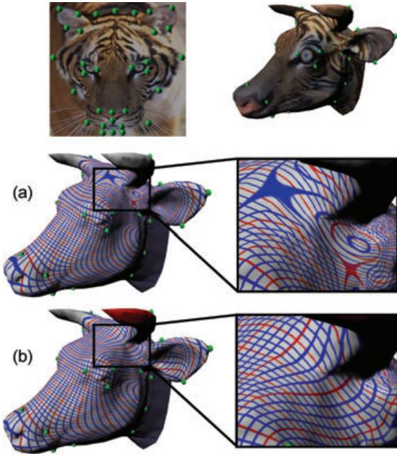
**Figure 2:** Constrained texture mapping using the Radial Basis Function (a); the resulting mapping is not bijective and the texture shows a foldover. Constrained texture mapping using our foldover-free image warping (b).
