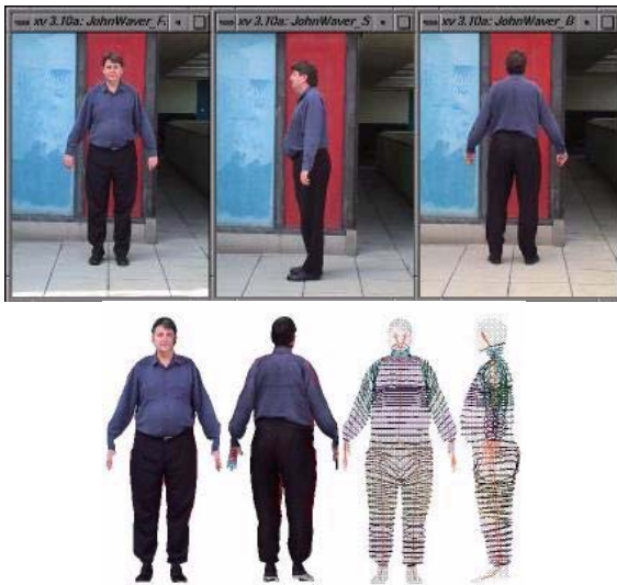
Figure 4. Image-based shape capture by Lee et al [19]. (up) Input images; (down) Reconstructed model.
