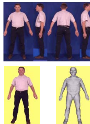
Figure 3. Image-based shape capture by Hilton et al[15]. (up) Input images; (down) Reconstructed model.
