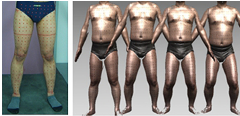
Fig. 1. Prior to the 3-D scan, we place color markers on the skin of the subject (left). Screenshot of 3-D laser scans of a subject at various poses (knee flexion angles of 0°, 30°, 45°, and 60°) (right).
