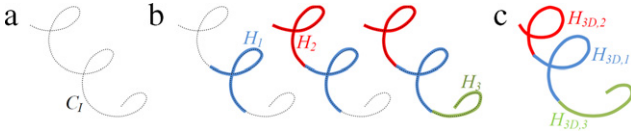
Fig. 1. Overview of the approach: the first step, which is shown in (b), consists of fitting a set of projected helix curves \{H_1, H_2, H_3\} to different parts of the input polygonal curve C_I as shown in (a). In the second step, which is shown in (c), the helices curves \{H_{3D,1}, H_{3D,2}, H_{3D,3}\} are computed in 3D from their projection \{H_1, H_2, H_3\} . Then, a fine fitting is performed to reduce the tangent discontinuity at the junctions of these helices.
